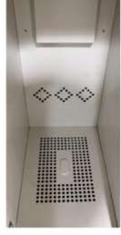
The air is sucked through the ventilation holes into the fan housing where it is blown into the surrounding room. A controller above the fan housing determines how much air goes to the exhaust air system and how much is to be circulated. Ventilation with circulating air is the fastest way to get wet clothes in lockers dry.
